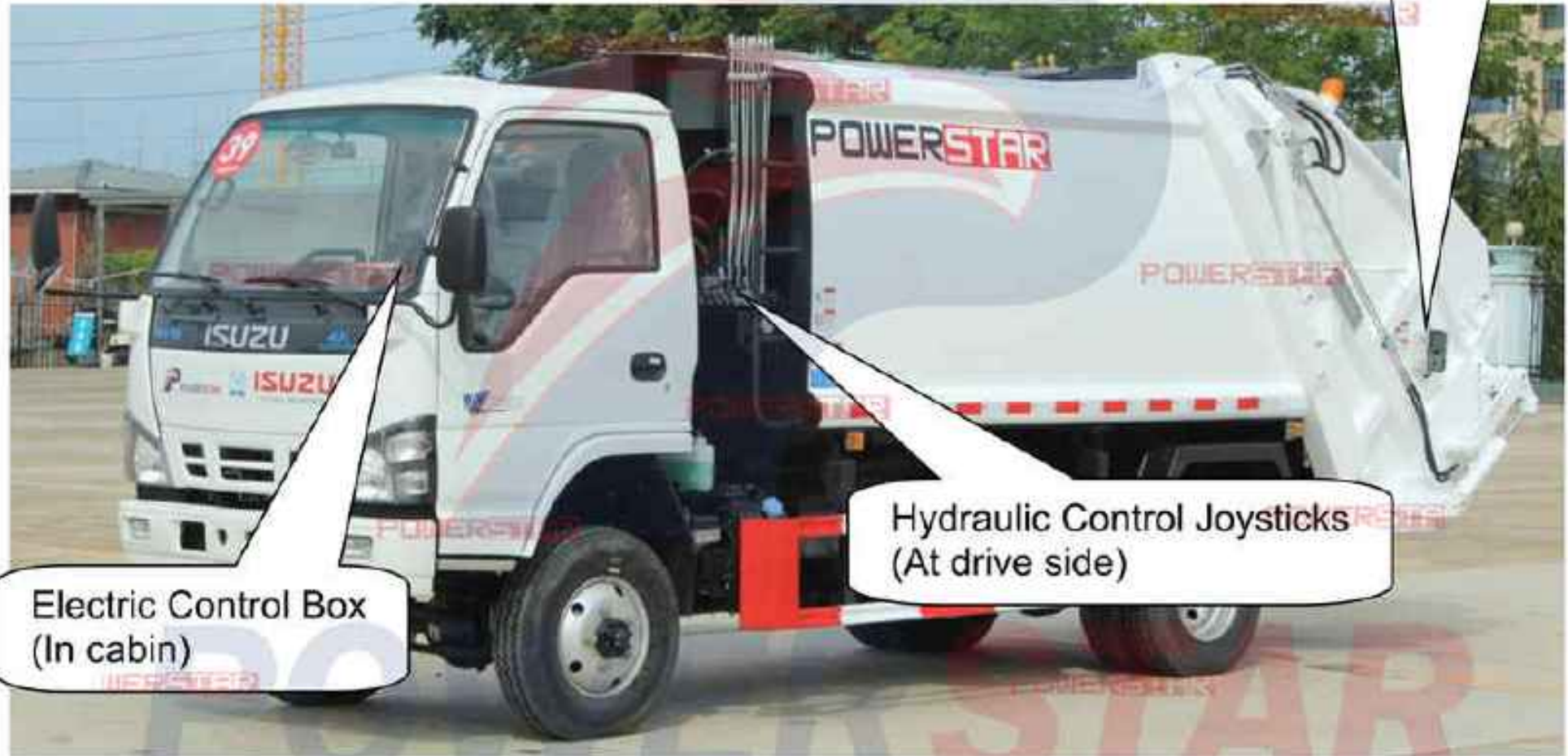
Front View: Hydraulic control system
